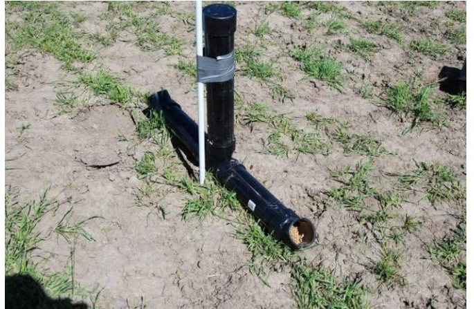
Figure 7. Inverted T bait station with spill guards.
