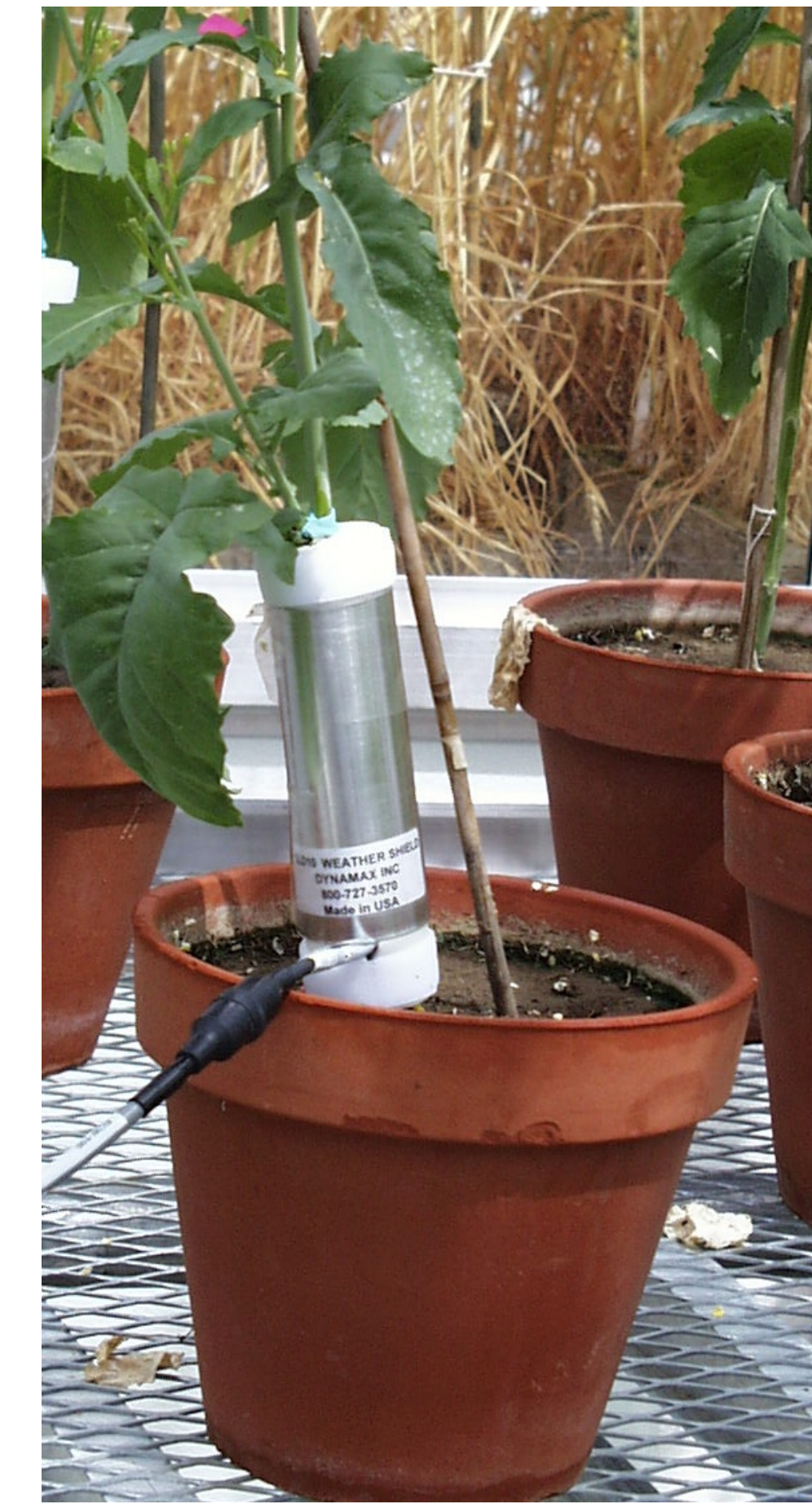
Fig. 2. Sap flow gauge installed on a canola plant in the greenhouse trial. Weather shield is installed to avoid external heat entering the system.
