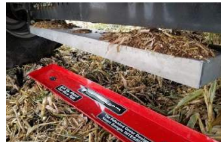
Figure 1. Remote controlled drop pan used to collect losses
