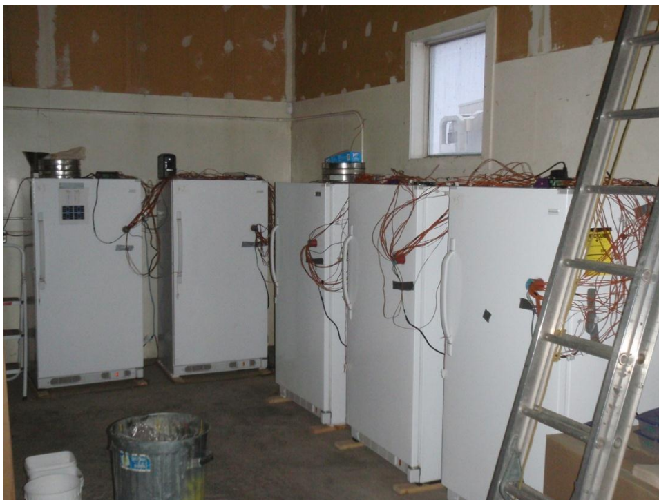
Figure 1. Five environmental chambers with thermocouples installed.
