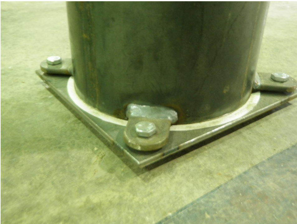
Figure 6. Compression testing container with removable bottom.
