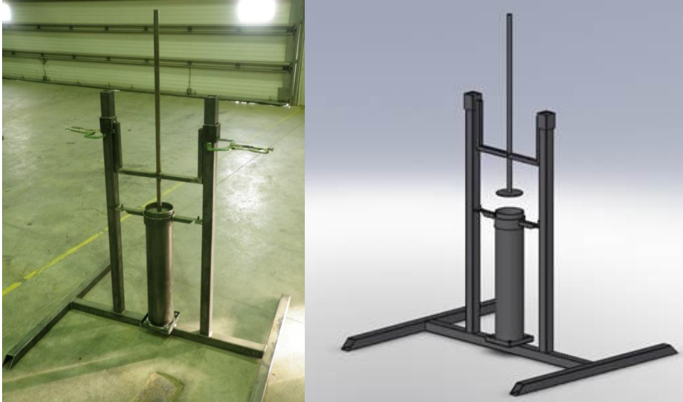
Figure 5. Canola compression test stand.
