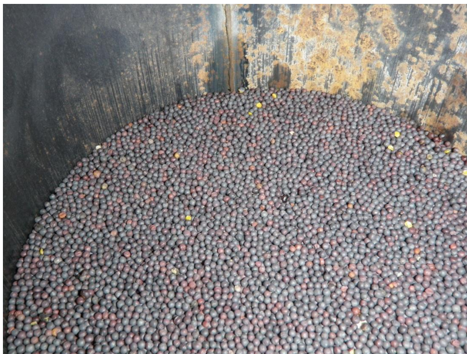
Figure 12. Deformed seeds at the top of the column against the plunger.
