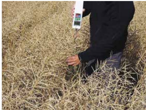
This tool measures the pod attachment strength.
