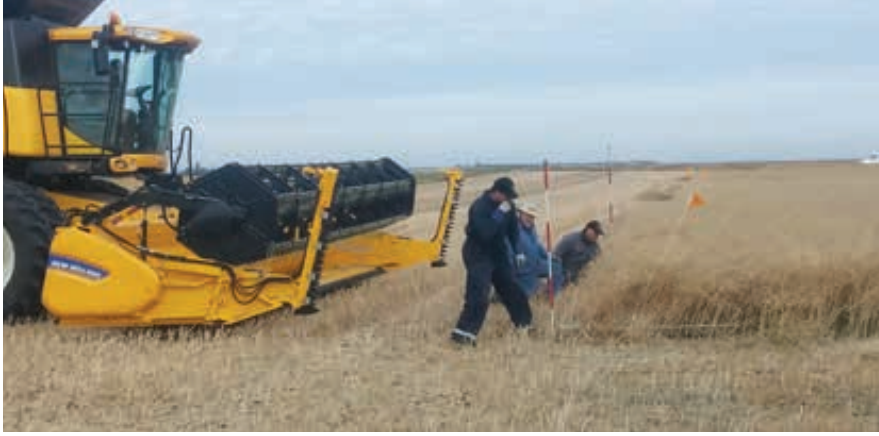
PAMI has just started a three-year header comparison study looking at yield, seed quality, header shatter loss, and environmental shatter loss for draper, rigid and extendable cutterbar headers as well as a swath-based system.
