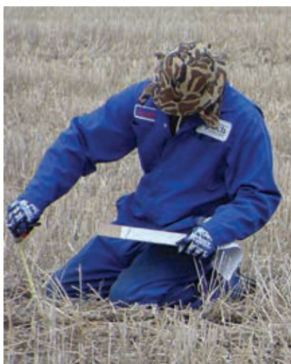
Researchers measure the seeding depth to see how canola seed placement varies by seeding speed and opener type.
