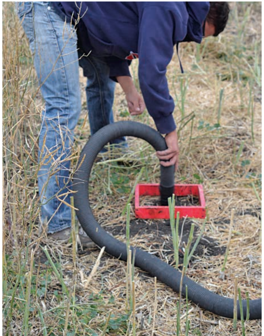
To measure harvest losses, all soil and crop debris, including dropped seeds, are vacuumed. Seed is then separated from the sample, and weighed.
