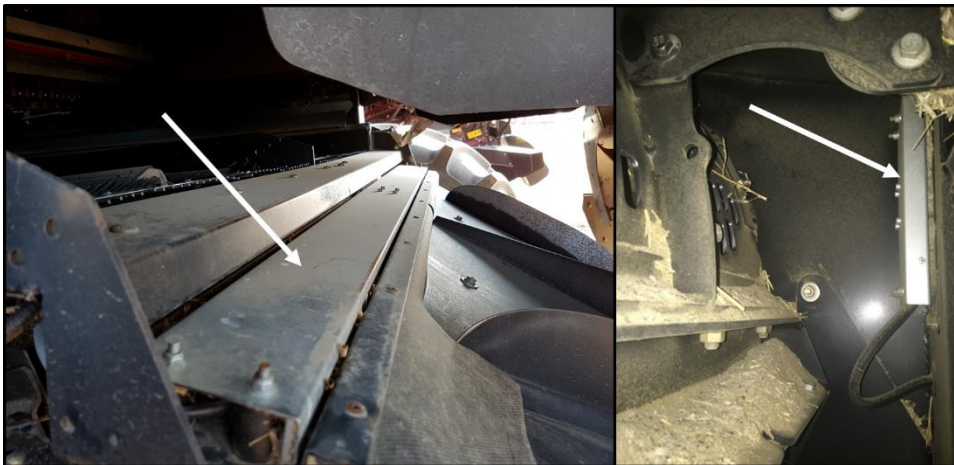
Figure 7. Cleaning shoe loss sensor (left) and separator loss sensor (right).
