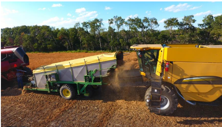
Figure 9. Collector top belt being unloaded into processor.
