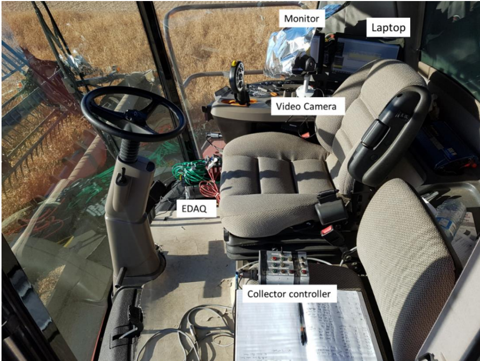
Figure 5. Test combine cab with data acquisition equipment labeled.
